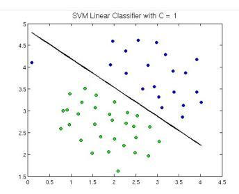
Here we can see a hyperplane which is separating green dots from the blue ones. A hyperplane is one dimension less than the ambient plane. E.g. in the above figure, we have 2 dimension which represents the ambient space but the lone which divides or classifies the space is one dimension less than the ambient space and is called hyperplane.
